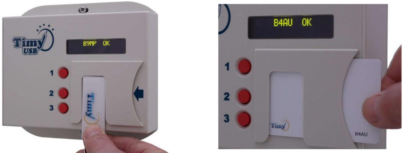
It is ideal for applications within a single site, with one or more clocking points or for those businesses where there is no power or network allowed or present on site. The Timy system uses 4 x standard AA alkaline batteries that hold about 20,000 clocking's and provides a very simple solution for data recovery via a USB key.
